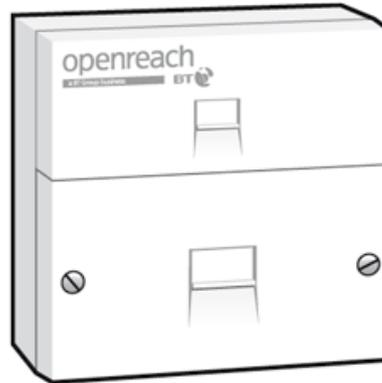
This is a filtered faceplate, identifiable by the two sockets. The top one is for broadband and the below is for telephone. A microfilter is not required with this type of faceplate.
